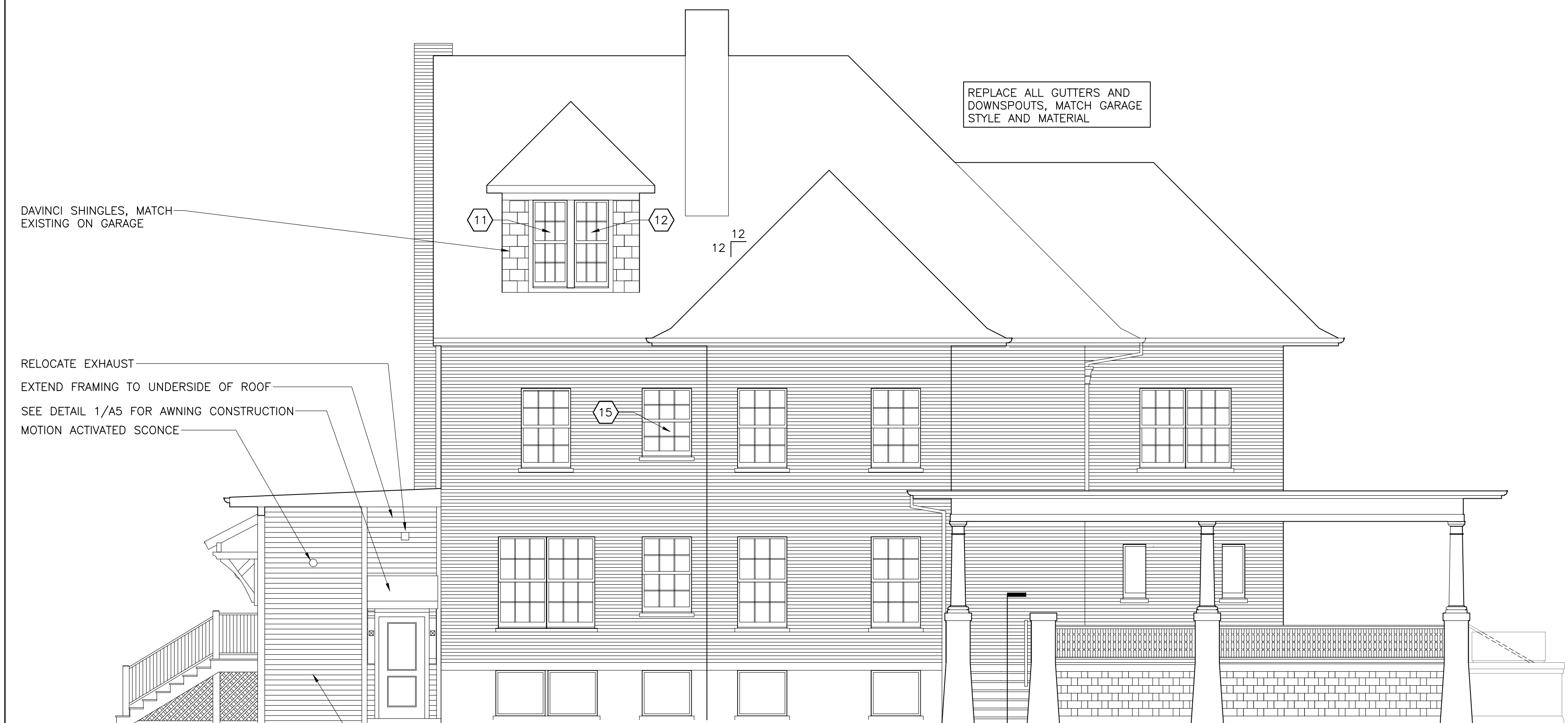
3 NORTH ELEVATION SCALE: 3/16" = 1'-0"
