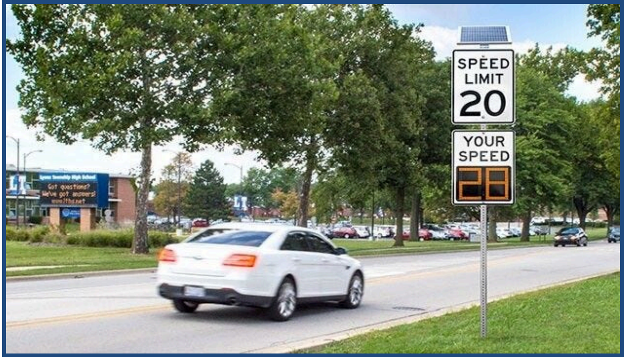
Sample of Permanent Radar Speed Sign
