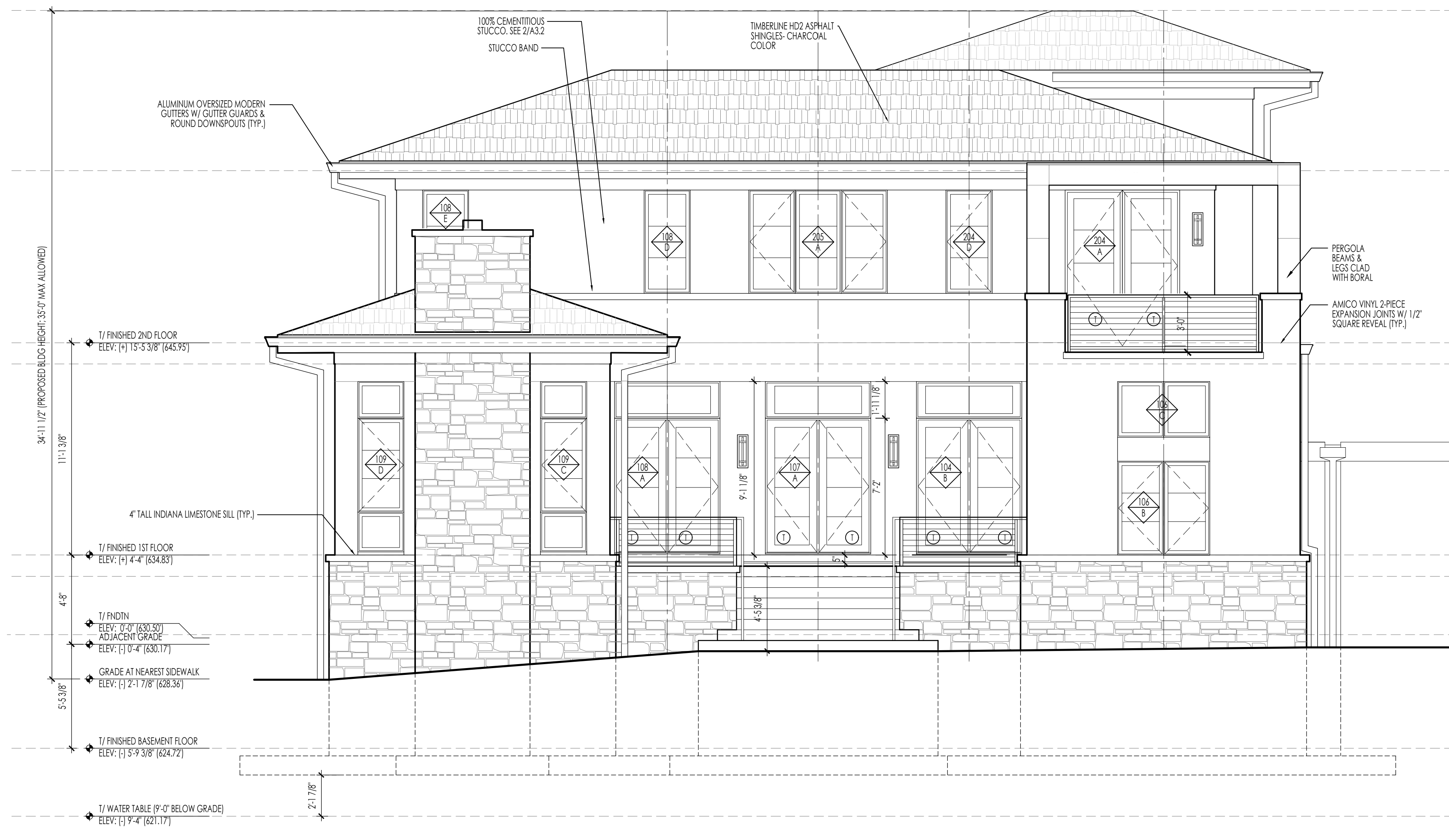
3 EXTERIOR ELEVATION - WEST A2.0 Scale: 1/4" = 1'-0"
