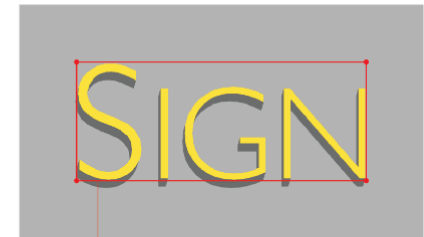
Measurement of sign area without backing
