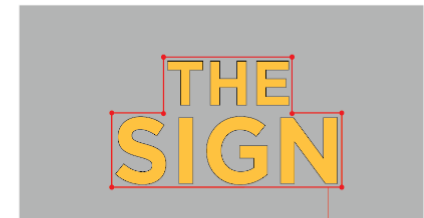
Measurement of sign area without backing
