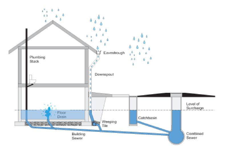
SEWER BACKUP can occur when the water level of the combined sewer in the street exceeds the basement elevation of an adjacent home with a gravity flow sewer connection.
